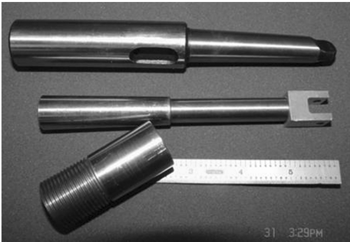
FIGURE 1 Simple slack adaptor components fabricated from a #2 Morse taper extension, as shown at the top.
